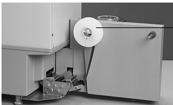
The first film goes on the reel closest to the processor
